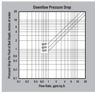
**PRESSURE DROP** — The graph above shows the expected pressure loss per foot of bed depth as a function of flow rate at various temperatures.
