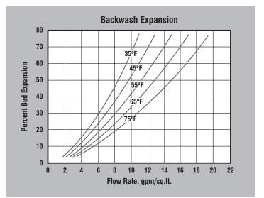
**BACKWASH** — After each cycle the carbon bed should be backwashed at a rate that expands the bed 30 to 50 percent. This will remove any foreign matter and reclassify the bed.The graph above shows the expansion characteristics of ProActive 20 x 50 SuperCat Coconut Shell Carbon.
